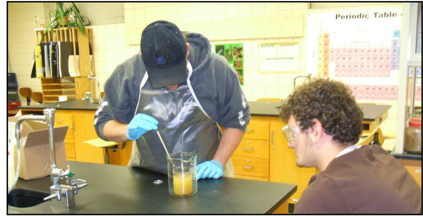
BRTC chemistry class conducts an analysis of early samples of mortar from the Rice - Upshaw House chimney and foundations for composition evaluation
